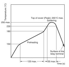
Note: Temperatures are given for the surface of the terminal.
